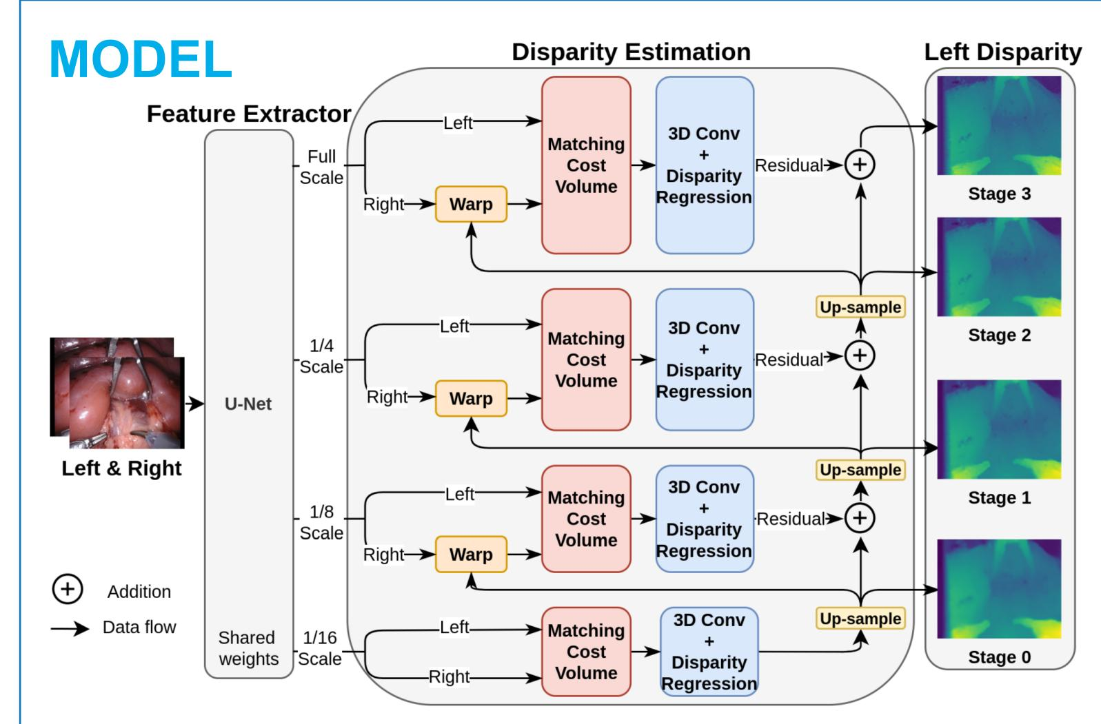
The architecture of our staged model. The input for both training and test phases is a pair of rectified stereo images. The outputs are four left disparity estimations. The input images are from the 2018 Robotic Scene Segmentation (RSS) dataset [3].
